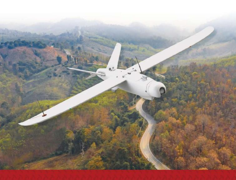
Includes high-performance daylight payload module with built-in video camera. Gyroscopically stabilised in two axes. Variable optical zoom. Night vision payload module with built-in thermal camera and fixed optical zoom.
