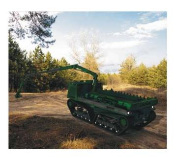
The Aardvark GEN2 is highly capable across a wide range of ground conditions and effectively delivers the ability to disrupt or destroy all anti-personnel and anti-vehicle landmines.
