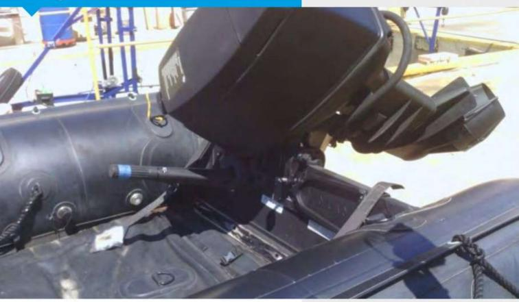
Safety Jet allows operators to change to a "pump jet" in less than 10 minutes. The Safety Jet allows for operation of the Raider Outboards in "brown" water where debris is present; beneficial for training whereby no moving parts of the engine can hurt the trainees if they should come in contact with the lower unit; protects the lower unit when beaching and can withstand minor contract with underwater obstacles. The user can switch back to a propeller within 10 minutes.
